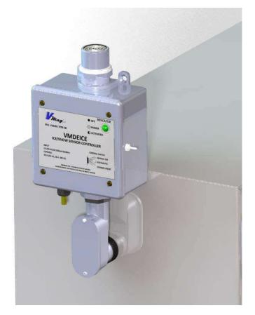
Prevents ice & snow accumulation on the motor assembly, lock assembly and reaction fin in the vicinity of the motor assembly when icing conditions exist. Can be retrofitted in the field or factory installed when ordered as an option.
