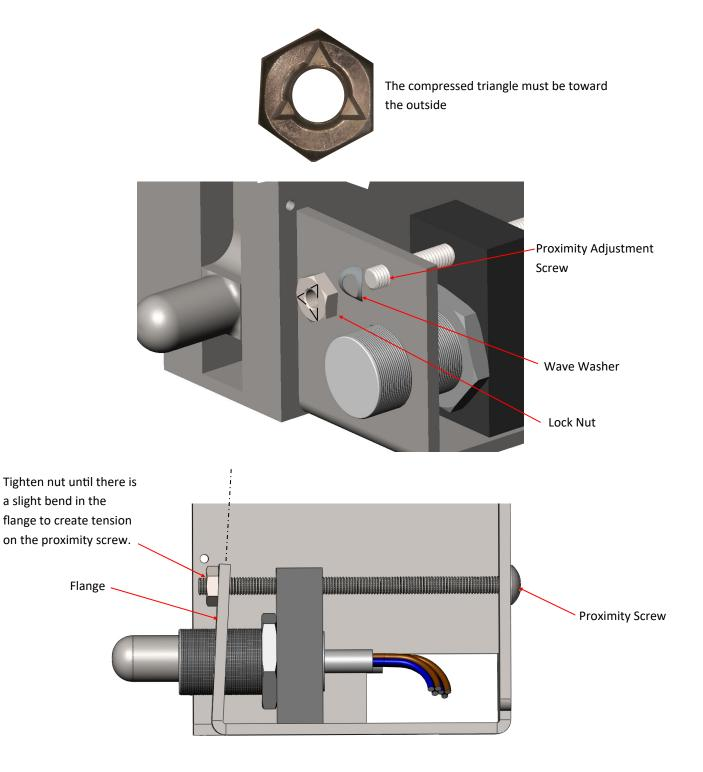
Re-install lock assembly and set the gap distance with the feeler gauge.
