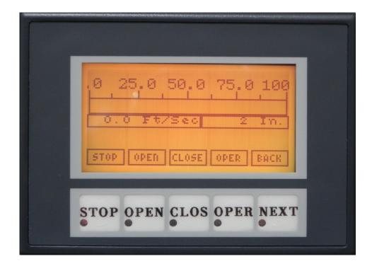
V KEEP ALIVE - Retains operator settings during brief disruptions in power or generator switching
