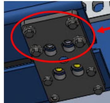
Loosen the four front bolts on each bracket. Do not loosen the rear bolts.
