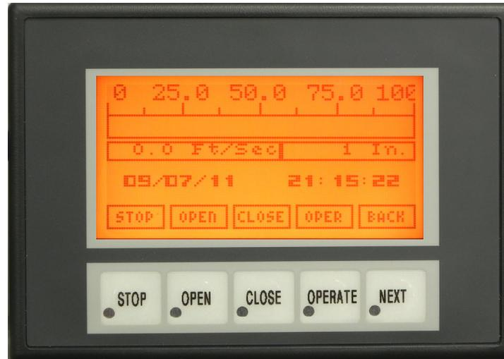
The V Programmer allows the technician to customize the gate operation to the user's preference and aid in troubleshooting. The programmer is not included with Vmag operators and should only be available to factory authorized installers and their trained customers.
