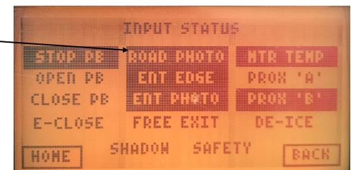
Any other input that is active will prevent normal operation and will require troubleshooting the related device. Card readers, keypads and free exit loop detectors will normally be connected into the **FREE EXIT** input. If more than one device is connected into the same input remove all devices from that input, then re-connect one device at a time until that input is highlighted indicating the defective device. *Continued.....*
