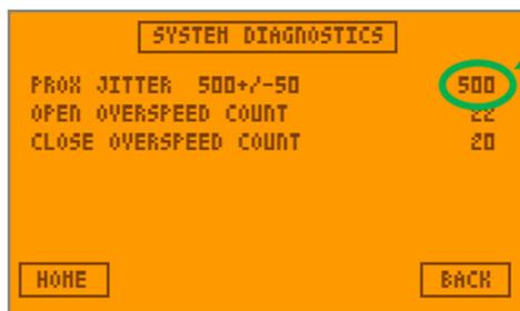
**Prox Jitter** value displays a variance between the proximity switches. This value should be as close to **500** as possible.
