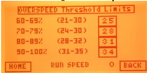
**OVERSPEED Threshold Limits** - If the gate speed exceeds the threshold limit an over speed condition is detected and will stop the gate.
