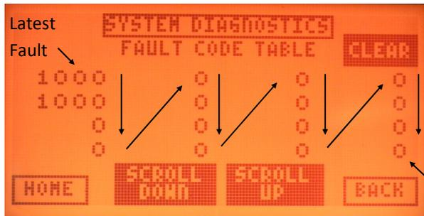
The **FAULT CODE TABLE** is in the **SYSTEM DIAGNOSTICS** page of the programmer.
