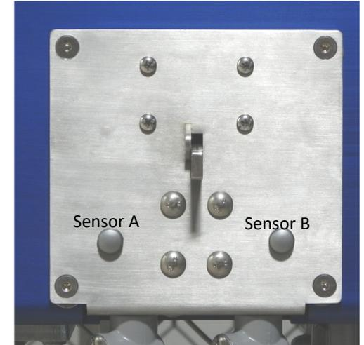
Re-check the **PROX JITTER** on the programmer. The value should be 500 +/- 2
