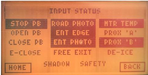
**INPUT STATUS** - Highlights active inputs. **STOP PB, ENTRAP & MTR TEMP** are normally activated.
