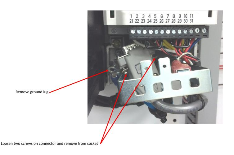
Gently pry connectors off with a small flat blade screwdriver
