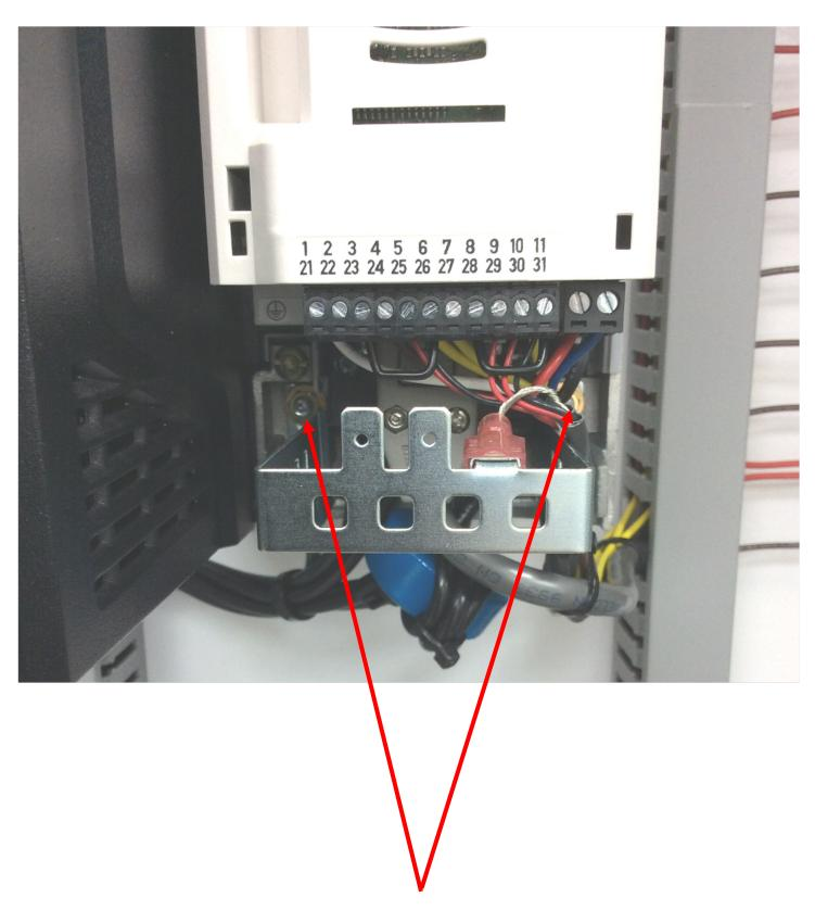
Remove two nuts using a 7mm socket
