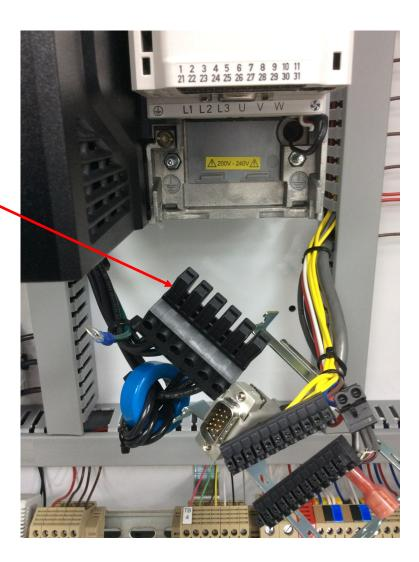
Gently remove power connector using a small flat blade screwdriver
