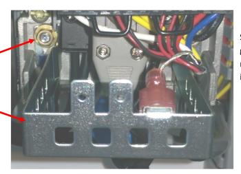
Slide the right side of the grounding bracket under right nut and tighten (nut not visible in this picture).
