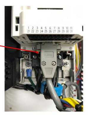
Slide the left side of the grounding bracket UNDER the ground lug and push up to the stud. Tighten nut.
